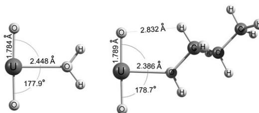
Figure 4. Structures calculated for [UO<sub>2</sub>(H<sub>2</sub>O)]<sup>+</sup> (left) and [UO<sub>2</sub>(*n*-PrOH)]<sup>+</sup> (right), using PBE/SDD/TZVP.
